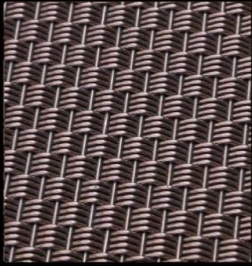
QKCWM-15 Warp Diameter:1.5mm Weft Diameter:2mm Warp Pitch:7mm Weft Pitch:8mm Weight:14.74kg/m 2 Opening Area:0%
