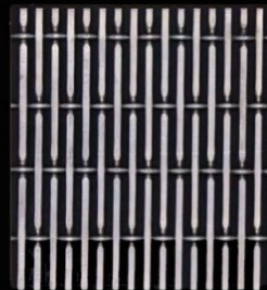
QKCWM-09 Warp Diameter:1.2x2mm Weft Diameter:2mm Warp Pitch:5mm Weft Pitch:5mm Weight:8.74kg/m 2 Opening Area:31%
