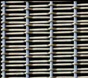
QKWWD-11 Cable Diameter:2.5mmx1 Rod Diameter:2mm Cable Pitch:6mm Rod Pitch:8mm Weight:9.8kg/m 2 Opening Area:44%
