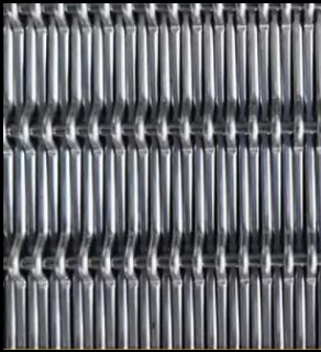
QKCWM-22 Warp Diameter: 2mm Weft Diameter: 1.5mm Warp Pitch: 17.5mm Weft Pitch: 1.5mm Weight: 11.67kg/m 2 Opening Area: 0%
