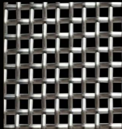
QKCWM-21 Warp Diameter:0.6x1.75mm Weft Diameter:0.6x1.75mm Warp Pitch:5mm Weft Pitch:5mm Weight:3.36kg/m 2 Opening Area:41%
