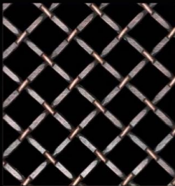
QKCWM-20 Warp Diameter:2mm Weft Diameter:2mm Warp Pitch:12.7mm Weft Pitch:12.7mm Weight:4kg/m 2 Opening Area:58.3%
