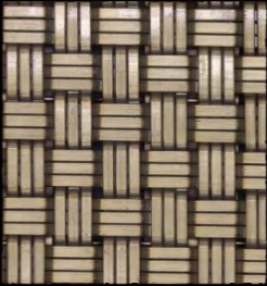
QKCWM-07 Warp Diameter:0.75x2mm Weft Diameter:0.75x2mm Warp Pitch: 15mm Weft Pitch:15mm Weight:6.5kg/m 2 Opening Area: 9.2%
